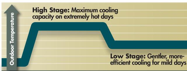
With its two-stage design, the 4SHP16LT makes the distinction between mild and extremely hot or cold days, using only the energy necessary to keep you comfortable.
